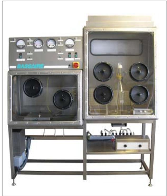
Within this facility temperature and pressure monitoring is indicated constantly and both isolators provide European 'Grade A' conditions. The construction even with the large access doors performed to a high integrity (a pressure loss of less than 50 Pascal's from a 1000 Pascal test pressure when corrected for temperature and ambient variations) above the medium integrity originally specified.
